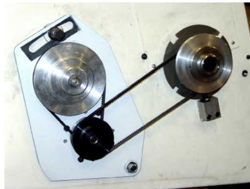
Figure 5.15 – Pulleys on high speed setting
