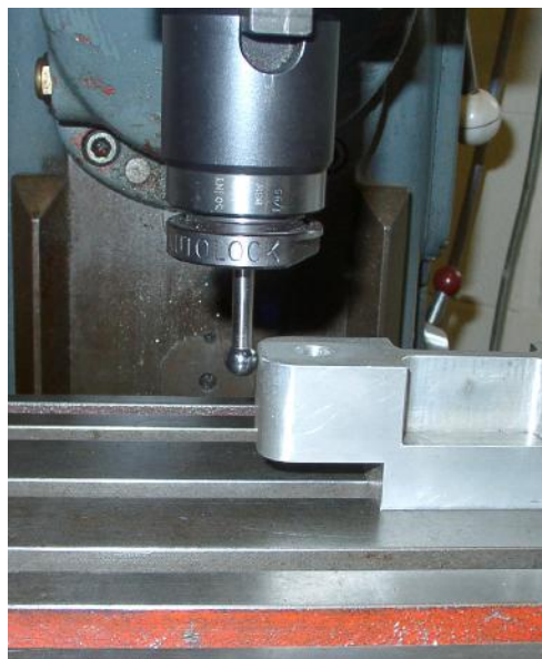
Figure 7.12 - Edge-finder in use on a mill
