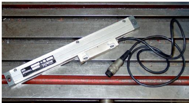
Figure 4.15 - Glass scale encoder (awaiting installation)
