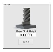
Tool 3 is ready to have a length offset applied. It will be the value that is shown in the Z DRO. To set this offset for Tool 3, the "Set Tool" button will be used. This is located to the right of the "Z Offset" set button in the Offsets tab.
