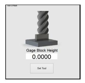
Unlike Tool 1 (the master tool), Tool 2 is going to have a length offset assigned to it. It will be the value that is in the Z DRO. To set this offset for Tool 2, the "Tool Offset" set button will be used. This is located to the right of the "Z Offset" set button in the Offsets tab.
