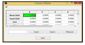
This can also be verified by opening the fixture table and looking at the Z column in the G54 row.
