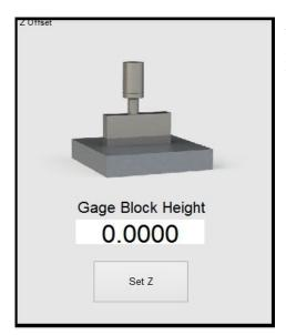
Next, set a fixture (G54) offset for Z. This will establish a reference surface on the Z axis so the Z offsets for tools 2-4 can be set later. So with Tool 1 on the surface of the stock, use the "Set Z" button from the Offsets Tab.
