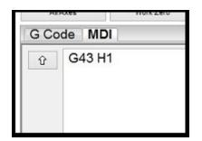
Once the tool change is complete in the MDI tab, enter G43 H1, and hit Cycle Start. This will activate the tool offset for tool 1. These commands can also be on the same line.
