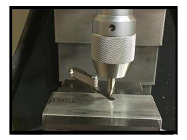
Tool 1 was loaded in to the tool holder and has been manually jogged down to the top of the piece of material that is slated to be machined. In the picture, a shim is used to finish bringing the tool down onto the work piece. This is used as an indicator to know when the tool begins to touch, and to avoid damaging the tool on the work piece.
