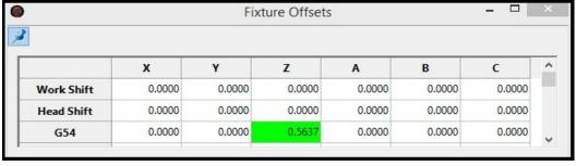
A glance at the "Current Z DRO" states that G54, or Z fixture offset, is zero. Opening the Fixture Offsets Table, you see that the Z
