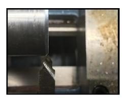
Jog Tool 3 into position to set the Z tool offset.
