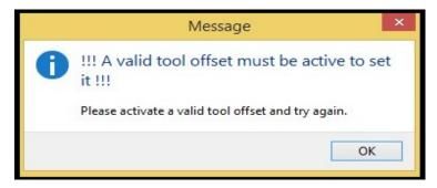
Because the Z tool offsets used in Mach4Lathe are simply a relationship between themselves, a fixture offset, and the master tool, referencing/homing the Z is not critical. If the machine has a limit or home switch wired for the Z axis, homing the Z upon start up will not interfere with setting offsets. However, if homing the Z is a habit continue to do it and proceed
