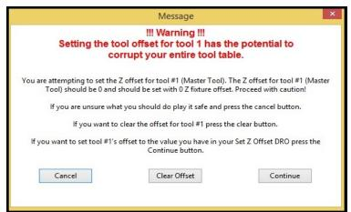
If "SET Z OFFSET" is clicked, while setting the fixture offset for Tool 1, the Master Tool, Mach4 will ask to continue with this action. The Z Offset for this tool should be zero.
