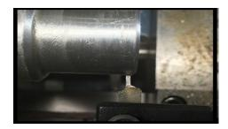
The offset in X should be set on the turned 1.0" diameter in the lathe (this value should still be in the SET X OFFSET DRO). With Tool 2 on the 1.0" diameter,
