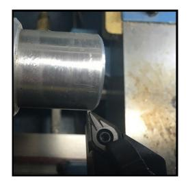
Tool 1 is loaded in the tool holder and has been used to turn a 1.0" diameter. When the cut is complete, X should not be moved. Move the tool off the part with the Z axis while the spindle is still turning.
