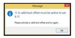
If the previous step is missed and a tool offset is not active, Mach4 will remind users to do so with this message box. If this shows up, the previous step (calling a tool and its offset) must be repeated.
