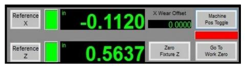
If the "Machine Pos Toggle" button is pressed, the Z DRO should now display .5637. This is the relationship between the Master Tool, Fixture Offset, and machine coordinates.
