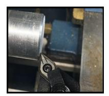
Tool 1 has been touched off the face of the work piece and is in position to set the fixture, or G54, offset.
