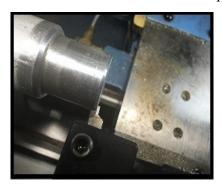
When setting the Master Tool, the "SET OFFSET Z" button was not used. A fixture offset was set, leaving zero for a value in the Tool 1's Z offset.
