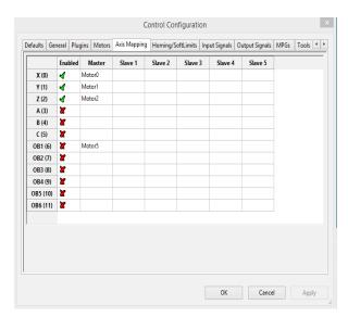
After the OB axis is set up, it needs to be assigned so it can be accessed by the THC Module.
